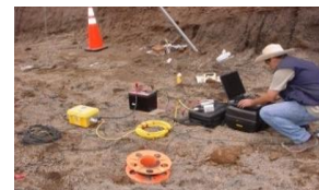
Fig. 4: Geophysical testing (seismic refraction and MASW) at the project site during planning and design phases.
